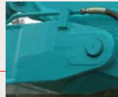
Integrated cast steel boom top
